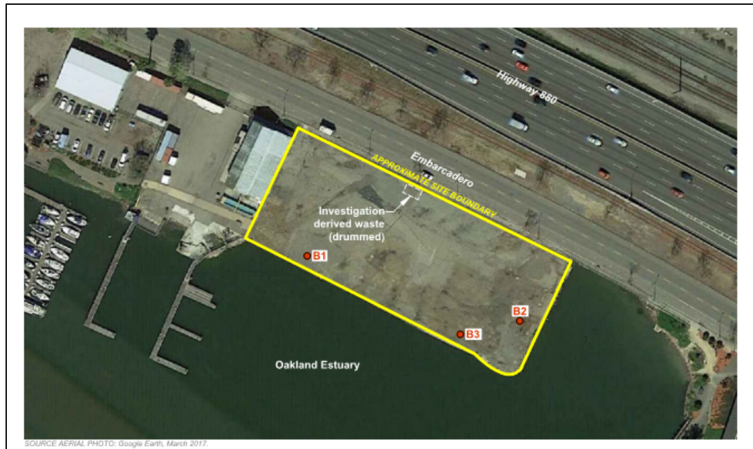
Figure 11: Geotechnical boring locations
